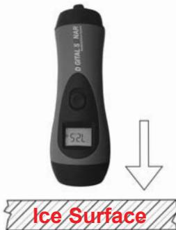
3. If there are any air pockets between the unit and ice, or the water below the ice, the unit will not work properly and will require you to try another spot, or cut a hole in the ice to use.
